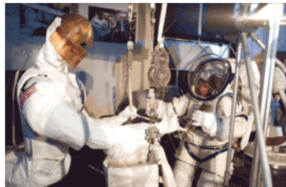
Robonaut working with astronaut Nancy Currie to build an aluminum truss. Photo courtesy of NASA.
